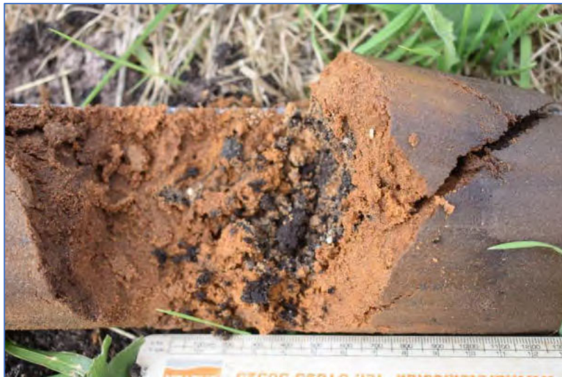
Plate 7: TP22 Probable wind blown sand at 2.5m below ground level
